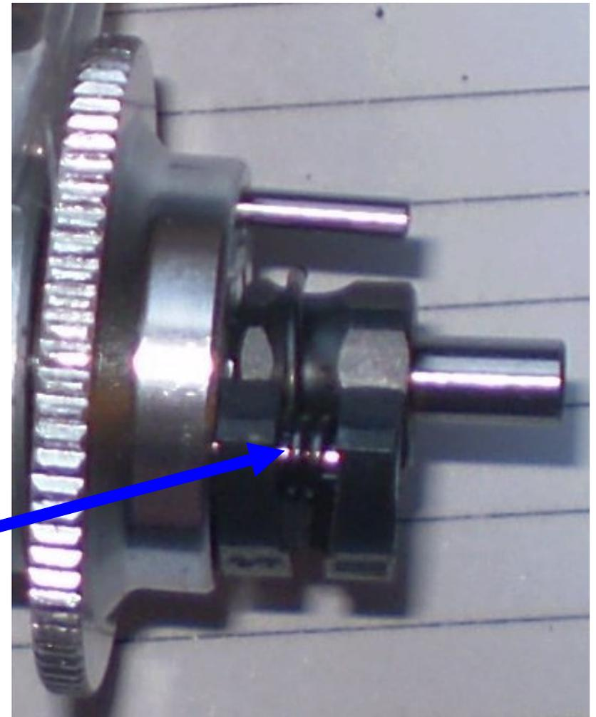
Note, the longer part of the spring wraps around flywheel securing nut
