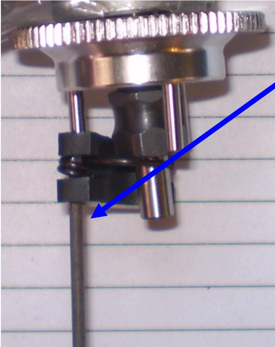
**Help – Clutch Assembly** The springs on the clutch shoes are very strong and difficult to assemble see photograph for the way in which we used a guide pin alternatively you can buy an Ansmann clutch installation too.
